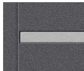
Double-sided embossing width 25 mm with inlay in INOX finish or painted black. The inlay may be placed either on one or on both sides. It is placed in embossing and flush with the leaf (STAMP) or boned to a flat leaf (LABEL).
