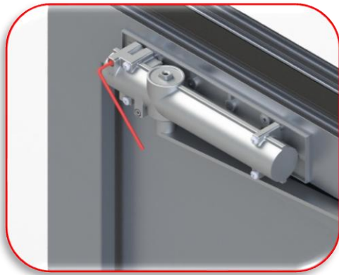
16. Adjust the closing speed using the screw labeled "2" with an Allen key.
