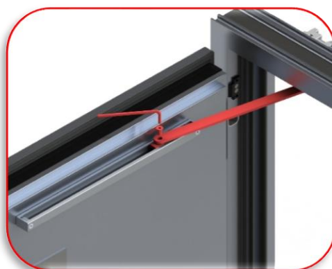
13. Secure the closer arm to the slider in the rail.
