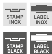
Double-sided embossing width 25 mm with inlay in INOX finish or painted black. The inlay may be placed either on one or on both sides. It is placed in embossing and flush with the leaf (STAMP) or bonded to a flat leaf (LABEL).
