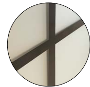
Black lines width 18 mm painted using screen printing technology
